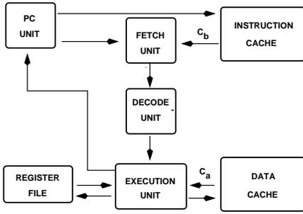
Figure 5: PDLX Microprocessor Block Diagram : top level view.
