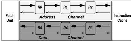
Figure 3: Channels between *Fetch Unit* and *Instruction Cache*
