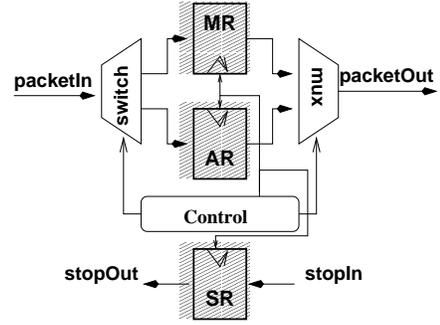
Figure 2: Relay Station Implementation
